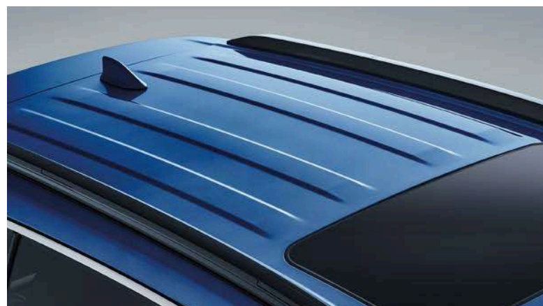
Roof Rails facilitate the easy installation of accessories such as a luggage carrier or roof rack cross bars.
