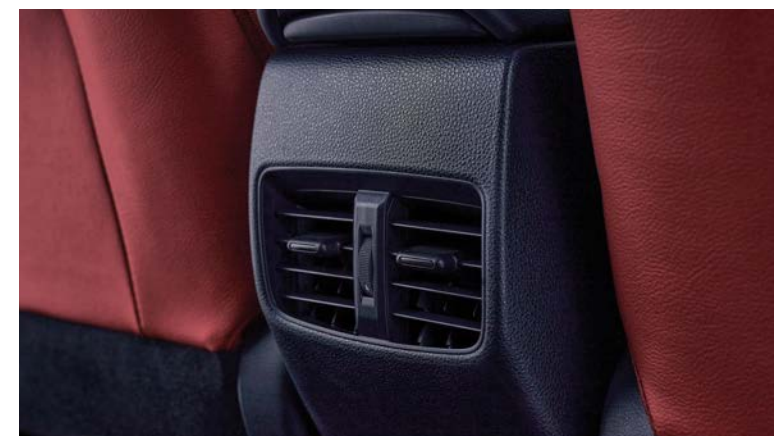
Rear Vents are located at the rear cabin to provide comfort to the passengers at the back.
