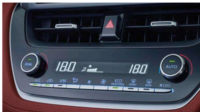
Dual Zone Auto Climate Control offers both the passenger and the driver to adjust the temperature according to their comfort.
