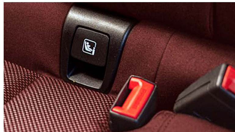
ISOFIX Child Restraint System is located at the rear that allows appropriate securing of child safety seat.
